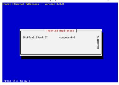
You will see this type of output for each compute node that is successfully identified by insert-ethers.
