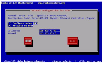
The above window is an example of how we configured the external network on one of our frontend machines.
